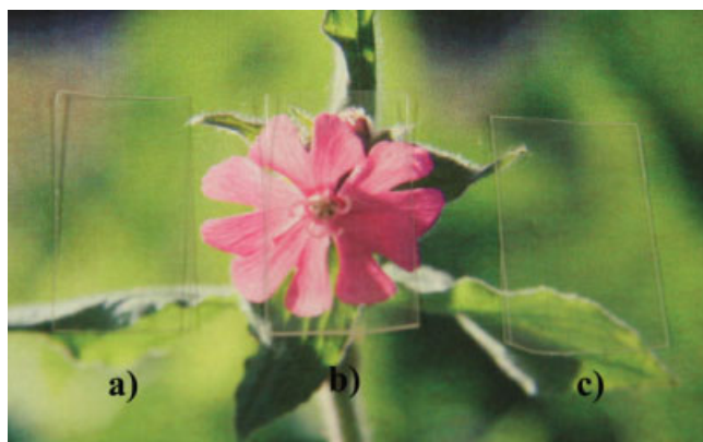
Figure 2 Visual comparison of the optical clarity of the produced materials. (a) CAB, (b) CAB/CNW, and (c) CAB/LS. [Color figure can be viewed in the online issue, which is available at www.interscience.wiley.com .]
