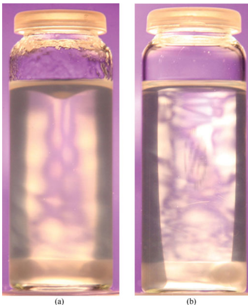
Figure 1 Flow birefringence of the cellulose nanowhiskers. (a) Dispersed in ethanol and (b) Dispersed in ethanol and dissolved CAB. [Color figure can be viewed in the online issue, which is available at www.interscience.wiley.com .]
